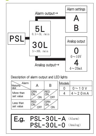
NOTE) Default setting of alarm output is 5L=2.5L/min · 30L=15.0L/min.
