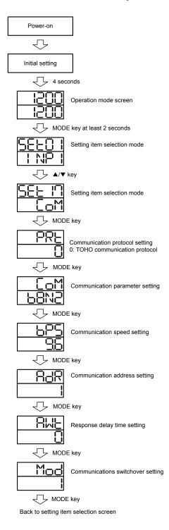
When the settings are over, press the MODE key at least 2 seconds to go back to the operation mode. The parameters indicated above are initial values.
