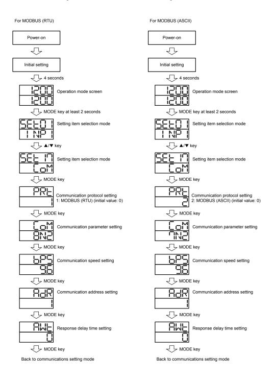
When the settings are over, press the MODE key at least 2 seconds to go back to the operation mode.
