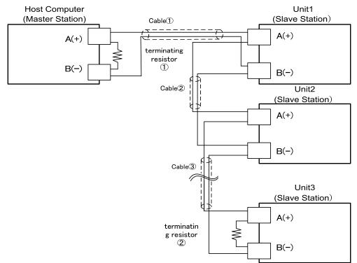
OAbove drawing shows example of connecting 1 to 3 slave stations to a master station.
