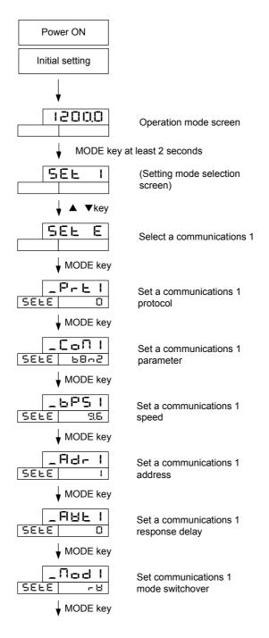
When the settings are over, press the MODE key at least 2 seconds to go back to the operation mode. The parameters indicated above are initial values.
