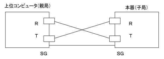
In actual practice, it is necessary to connect the CS (enable communications) in the connector to the ER (data terminal ready), and the RS (request communications) to the DR (data set ready) to the CD (detect the reception carrier).
