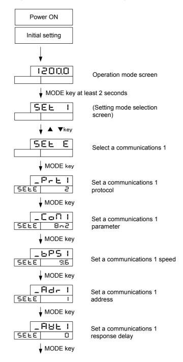
When the settings are over, press the MODE key at least 2 seconds to go back to the operation mode. The parameters indicated above are initial values.
