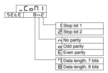
\* The ASCII mode settings come only in three types:  $\Box_{\Box} \ge \Box_{\Box} \ge \Box_{\Box} \ge \Box_{\Box} \ge \Box_{\Box}$ . The RTU mode settings come only in three types:  $\Box_{\Box} \ge \Box_{\Box} = \Box_{\Box} \ge \Box_{\Box} = \Box_{\Box} \ge \Box_{\Box} = \Box_{\Box} =$
