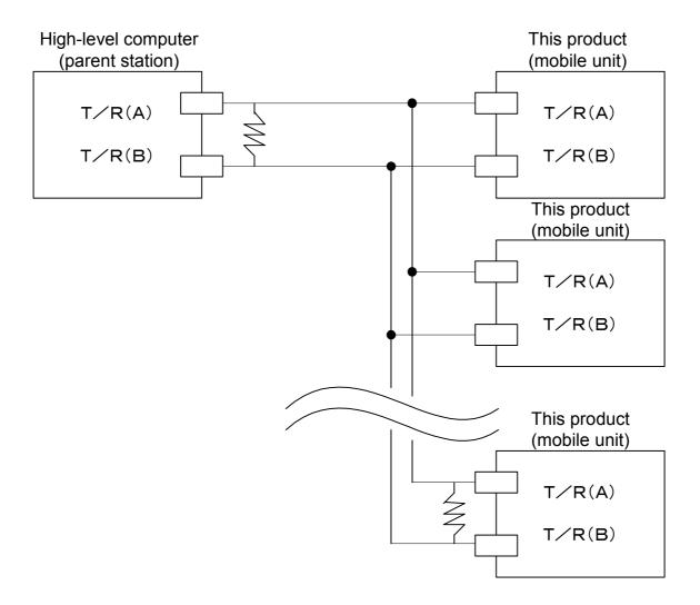
Install an end of line resistor at both of the farthest devices in the parent station and the mobile unit. For a resistance value, use one that matches the characteristic impedance of the cable. Provided that the synthesis is set to at least  $75\Omega$ .
