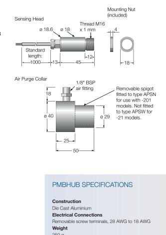
Die Cast Aluminium Electrical Connections Removable screw terminals, 28 AWG to 18 AWG Weight 250 g Environmental Rating IP65 Enclosure Dimensions Same as PM180
