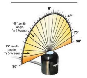
Directional, or cosine, response is defined as the measurement error at a specific angle of radiation incidence. Error for JMQ series quantum meters is approximately  $\pm$  2 % and  $\pm$  5 % at solar zenith angles of 45° and 75°, respectively.
