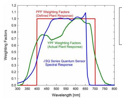
Radiation weighting factors for PPF (defined plant response to radiation), YPF (measured plant response to radiation), and quantum sensors (sensor sensitivity to different wavelengths of radiation).
