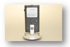
The AL-210 leveling plate is recommended for use with the JMQ-100.
