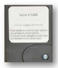
Sensor model number and serial number are located on a label on the backside of the handheld meter.
