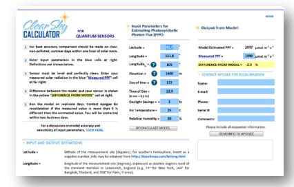
Clear Sky Calculator for quantum sensors. Site data are input in blue cells in middle of page and an estimate of PPF is returned on right-hand side of page.
