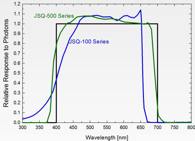
Mean spectral response measurements of six replicate JSQ-100 and JSQ-500 series quantum sensors. Spectral response measurements were made at 10 nm increments across a wavelength range of 300 to 800 nm in a monochromator with an attached electric light source. Measured spectral data from each quantum sensor were normalized by the measured spectral response of the monochromator/electric light combination, which was measured with a spectroradiometer.
