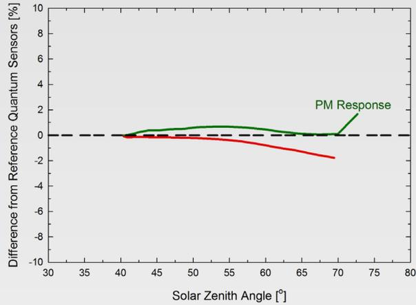
Mean cosine response of seven JSQ-500 quantum sensors. Cosine response measurements were made on the rooftop of the our building in Logan, UT. Cosine response was calculated as the relative difference of JSQ-500 quantum sensors from the mean of replicate reference quantum sensors (models LI-190 and LI-190R, PQS 1). The red data are AM measurements; the green data are PM measurements.
