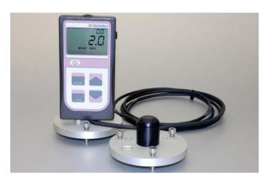
The ultraviolet meter measures and displays instantaneous readings of the ultraviolet radiation between 250 and 400 nanometers (nm) in µmol m<sup>-2</sup> s<sup>-1</sup> (micromoles of photons per square meter per second) or Watts. The selfcleaning dome-shaped head of the JMU-200 prevents water accumulation. The sensor head is potted solid to prevent internal condensation in humid environments.
