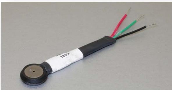
Sensor model number, serial number, and production date are located on a label between the sensor and pigtail lead wires.
