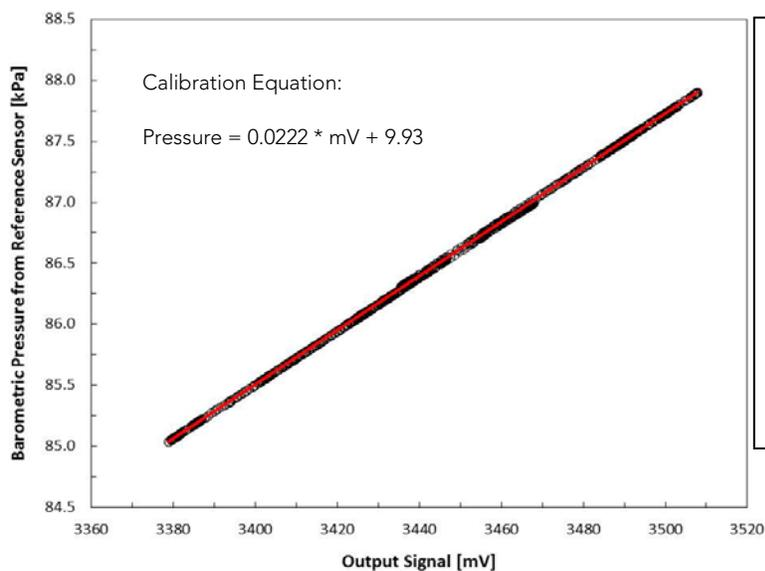
Example of JSB-100 barometric pressure sensor calibration
