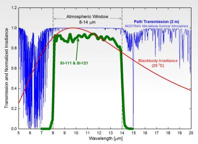
Spectral response of JSI series infrared radiometers. Spectral response (green line) is determined by the germanium filter and corresponds closely to the atmospheric window of 8 -14  $\mu$ m, minimizing interference from atmospheric absorption/ emission bands (blue line) below 8  $\mu m$  and above 14 µm. Typical terrestrial surfaces have temperatures that yield maximum radiation emission within the atmospheric window, as shown by the blackbody curve for a radiator at 28 C (red line).
