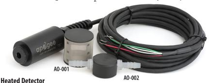
The protective membrane in front of the oxygen sensor can be heated to prevent water from condensing on the membrane and blocking the diffusion path. The heater is typically used when sensors are deployed in soil or compost where relative humidity is close to 100 %.
