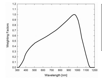
Spectral response estimate of silicomcellpyranometers. Spectral response was estimated by multiplying the spectral response of the photodiode, diffuser, and adhesive. Spectral response measurements of diffuser and adhesive were made with a spectrometer, and spectral response data for the photodiode were obtained from the manufacturer.
