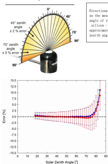
Cosine Response of Apogee JSP Series Pyranometers
