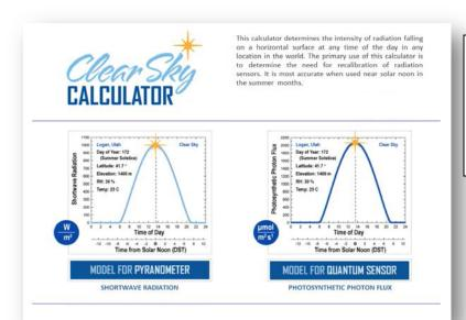
Homepage of the Clear Sky Calculator. Two calculators are available: one for quantum sensors (PPF) and one for pyranometers (total shortwave radiation).
