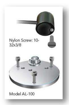
To minimize azimuth error, the sensor should be mounted with the cable pointing toward true north in the northern hemisphere or true south in the southern hemisphere. Azimuth error is typically less than 1 %, but it is easy to minimize by proper cable orientation.
