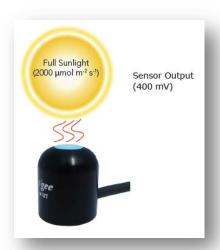
Example of PPF measurement with an quantum sensor. Full sunlight yields a PPF on a horizontal plane at the Earth's surface of approximately 2000  $\mu mol~m^{-2}~\bar{s}^1$ . This yields an output signal of 400 mV. The signal is converted to PPF by multiplying by the calibration factor of 5.00-2 $\mu mol~m~s^{-1}$  per mV.
