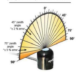
Directional, or cosine, response is defined as the measurement error at a specific angle of radiation incidence. Error for JSQ series quantum sensors is approximately  $\pm$  2 % and  $\pm$  5 % at solar zenith angles of 45° and 75°, respectively.
