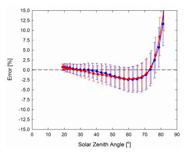
Mean cosine response of twenty-three JSQ series quantum sensors (errorbars represent two standard deviations above and bebw mean). Cosine response measurements were made by direct side-by-side comparison to the mean of four reference thermopile pyranometers, with solar zenith angle-dependent factors applied to convert total shortwave radiation to PPF. Blue points represent the AM response and red points represent the PM response.
