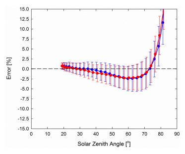
Mean cosine response of twenty-three JSQ series quantum sensors *error bars* represent two standard deviations above and below mean). Cosine response measurements were made by direct side-by-side comparison to the mean of four reference thermopile pyranometers, with solar zenith angle-dependent factors applied to convert total shortwave radiation to PPF. Blue points represent the AM response and red points represent the PM response.
