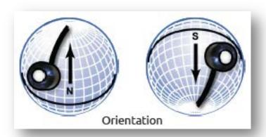
In addition to orienting the cable to point toward the nearest pole, the sensor should also be mounted such that obstructions (e.g., weather station tripod/tower or other instrumentation) do not shade the sensor. Once mounted, the green cap should be removed from the sensor. The green cap can be used as a protective covering for the sensor, when it is not in use.
