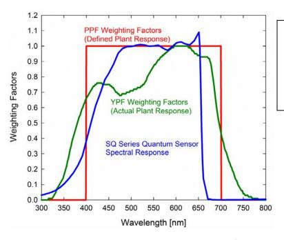
Radiation weighting factors for PPF (defined plant response to radiation), YPF (measured plant response to radiation), and JSQ Series quantum sensors (sensor sensitivity to different wavelengths of radiation).
