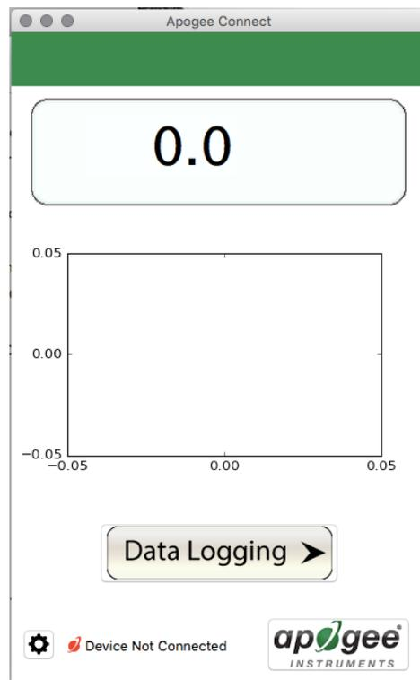
Plug the sensor into a USB port and allow some time for the sensor to automatically establish communication with the software. Once established, the message in the lower left corner will display "Device Connected Model: SN ####" and real-time shortwave radiation readings will update on the screen. Moving the sensor closer to a light source should increase the readings, while blocking all light from the sensor should drop the reading to zero.
