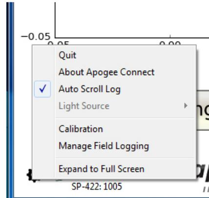
Clicking **'Calibration'** will display the factory calibrated multiplier and offset values. These values are saved in firmware and can be recovered by clicking the 'Recover Original' button. Deriving a new calibration multiplier and offset is accomplished by clicking the 'Recalibrate' button. This is applicable if users want to calibrate the sensor to their own specific light source. Note that a reference value of the light source is required to complete a recalibration.
