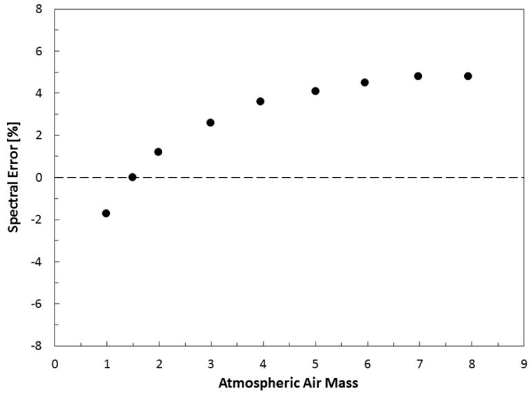
Spectral error for JSP series pyranometers as a function of atmospheric air mass, assuming calibration at an air mass of 1.5.
