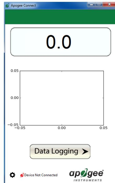
Plug the sensor into a USB port and allow some time for the sensor to automatically establish communication with the software. Once established, the message in the lower left corner will display "Device Connected SN: ####" and real-time shortwave radiation readings will update on the screen. Moving the sensor closer to a light source should increase the readings, while blocking all light from the sensor should drop the reading to zero.
