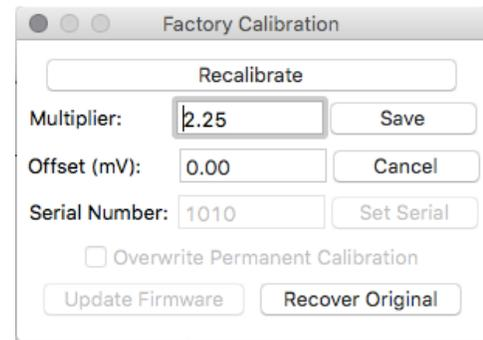
After clicking the 'Recalibrate' button the user will be prompted to cover the sensor. Place a dark cap over the sensor and wait for the real-time shortwave radiation reading to settle at zero. Click OK.
