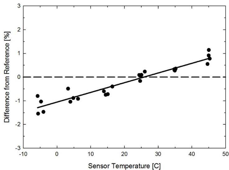
Mean temperature response of four the silicon-cell pyranometers. Temperature response measurements were made at approximately 10 C intervals across a temperature range of approximately -10 to 50 C under sunlight. Each pyranometer had an internal thermistor to measure temperature. At each temperature set point, a reference blackbody pyranometer was used to measure solar intensity.
