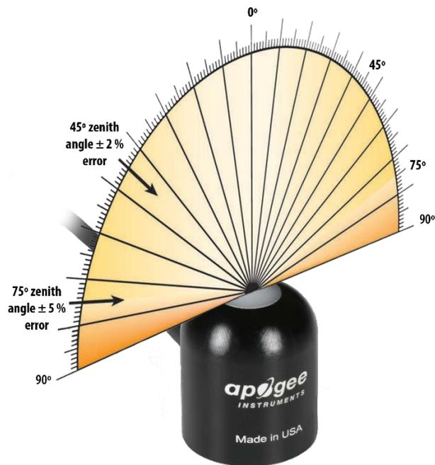
Directional, or cosine, response is defined as the measurement error at a specific angle of radiation incidence. Error for the silicon-cell pyranometers is approximately  $\pm 2\%$  and  $\pm 5\%$  at solar zenith angles of  $45^\circ$  and  $75^\circ$ , respectively.
