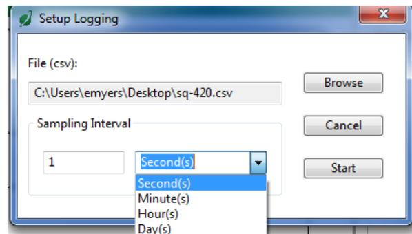
The data logging window will start to update at the specified sampling interval and display the Timestamp and Data Value. At the same time, data will be written to the csv file. Note that if the csv file is open in another program new data will not be saved to it.
