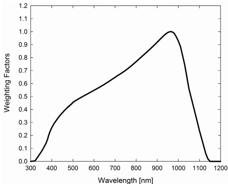
Spectral response estimate of the silicon-cell pyranometers. Spectral response was estimated by multiplying the spectral response of the photodiode, diffuser, and adhesive. Spectral response measurements of diffuser and adhesive were made with a spectrometer, and spectral response data for the photodiode were obtained from the manufacturer.
