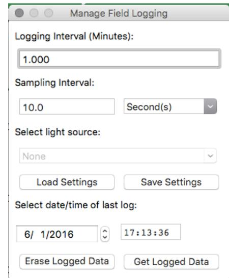
Set the sampling interval in minutes or seconds. The sampling interval is how often a measurement is taken and logging interval is how often the data is saved. The logged data is the average of the samples. The logging interval must be evenly divided by the sampling interval. For example if the logging interval is 5 minutes and the sampling interval is 2 minutes it causes an error. But a sampling interval of 1 minute is acceptable.
