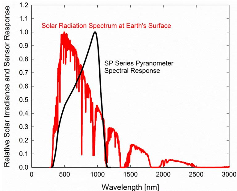
Spectral response of JSP series pyranometers compared to solar radiation spectrum at Earth's surface. Silicon-cell pyranometers, such as JSP series, are only sensitive to the wavelength range of approximately 350-1100 nm, and are not equally sensitive to all wavelengths within this range. As a result, when the spectral content of solar radiation is significantly different than the spectrum that silicon-cell pyranometers were calibrated to, spectral errors result.
