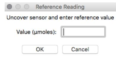
The multiplier and offset values will automatically calculate and update in the appropriate field. Be sure to click 'Save' to retain the new multiplier and offset.
