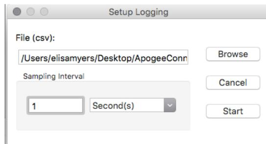
The data logging window will start to update at the specified sampling interval and display the Timestamp and Data Value. At the same time, data will be written to the csv file. Note that if the csv file is open in another program new data will not be saved to it.
