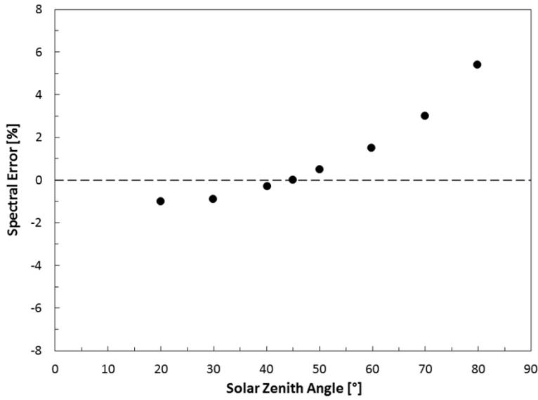
Spectral error for JSP series pyranometers as a function of solar zenith angle, assuming calibration at a zenith angle of 45°.
